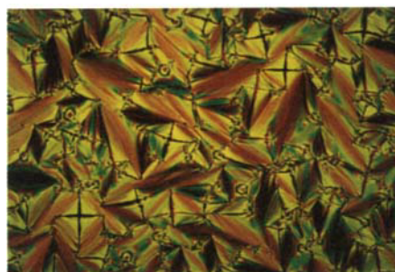
Figure 7. Photomicrographs between crossed polarizers of compound 5d : smectic A phase at 248°C (magnification \times 400 ).
